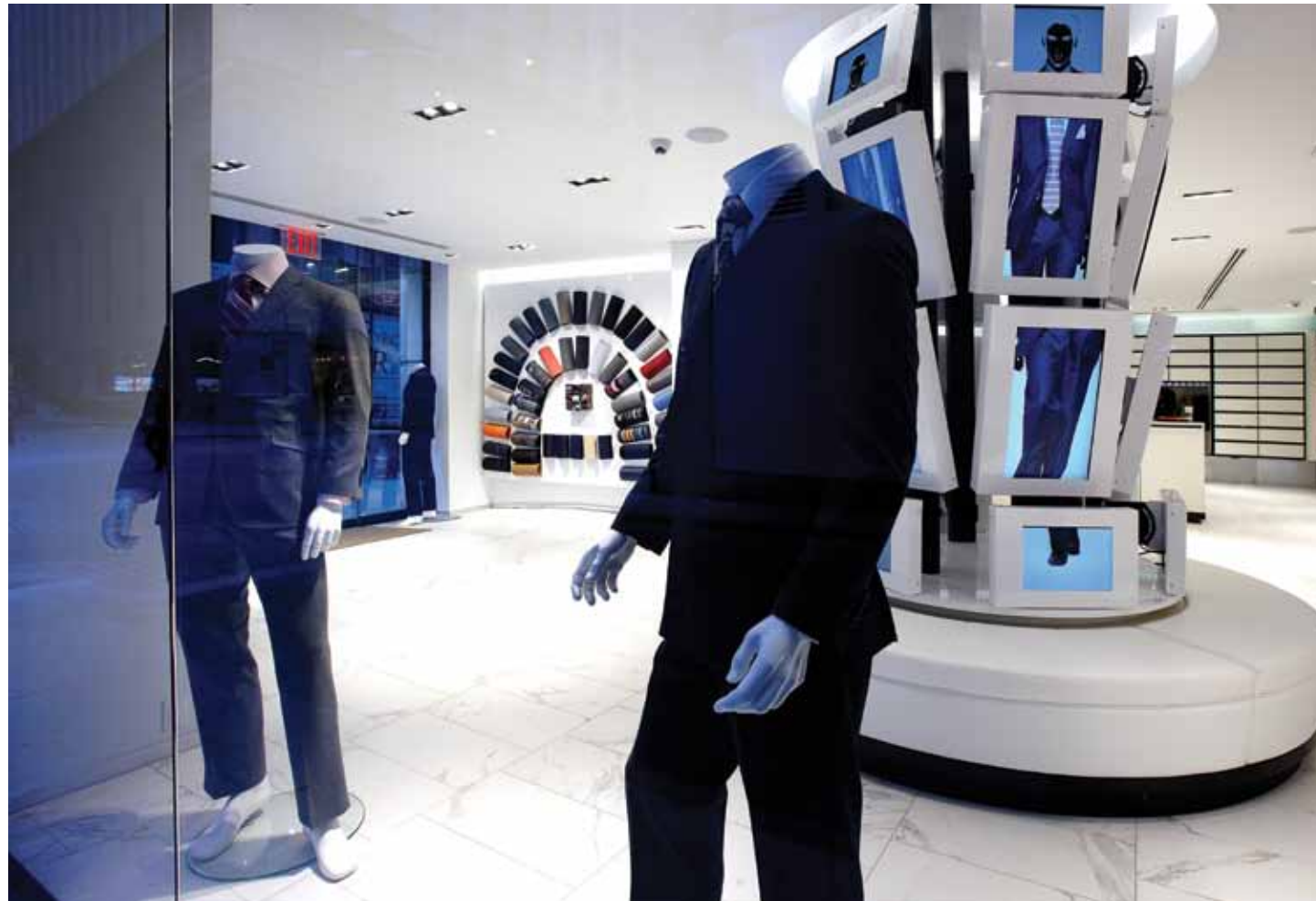
Customers can design their own suits in My.Suit's "design studio." Metal halide track heads recessed in ceiling slots provide ambient illumination and highlight a wall of fabric "pods." Topped with LED cove, the TV tower displays moving imagery for design inspiration.
