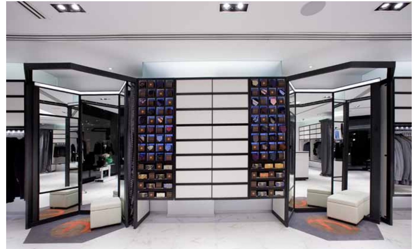
The fitting areas were inspired by a bridal shop. Lighted by metal halide downlights, they combine three functions—three-way mirror, dressing room and measuring station. The custom modular cabinets are illuminated from within and above by LEDs.
